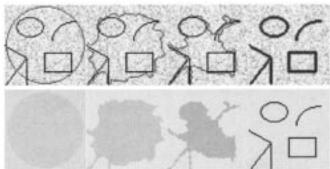
Fig. 6. Detection of lines and curves not necessarily closed. Size =  $64 \times 64$ ,  $\phi_0(x, y) = -\sqrt{(x-32.5)^2 + (y-32.5)^2} + 30$ ,  $\mu = 0.02 \cdot 255^2$ , no reinitialization, cpu = 2.88 s.
