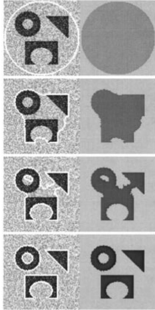
Fig. 4. Detection of different objects from a noisy image, with various shapes and with an interior contour. Left:  $u_0$  and the contour. Right: the piecewise-constant approximation of  $u_0$ . Size =  $100 \times 100$ ,  $\phi_0(x, y) = -\sqrt{(x - 50.5)^2 + (y - 50.5)^2} + 48.5$ ,  $\mu = 0.1 \cdot 255^2$ , no reinitialization, cpu = 4.60 s.
