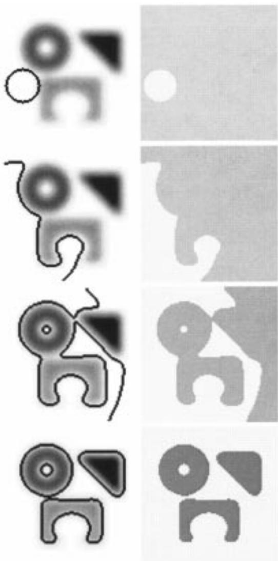
Fig. 5. Detection of three blurred objects of distinct intensities. Size =  $100 \times 100$ ,  $\phi_0(x, y) = -\sqrt{(x-15)^2 + (y-60)^2} + 12$ ,  $\mu = 0.01 \cdot 255^2$ , no reinitialization, cpu = 48.67 s.
