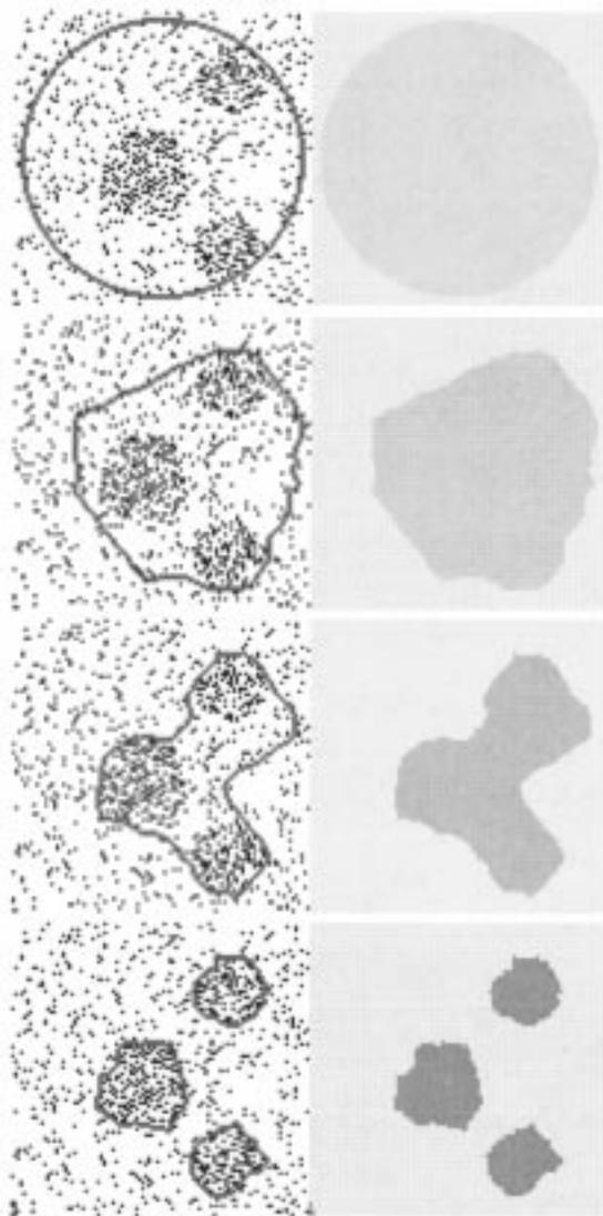
Fig. 10. Detection of a simulated minefield, with contour without gradient. Size =  $100 \times 100$ ,  $\phi_0(x, y) = -\sqrt{(x - 50.5)^2 + (y - 50.5)^2} + 47$ ,  $\mu = 0.2 \cdot 255^2$ , no reinitialization, cpu = 144.81 s.
