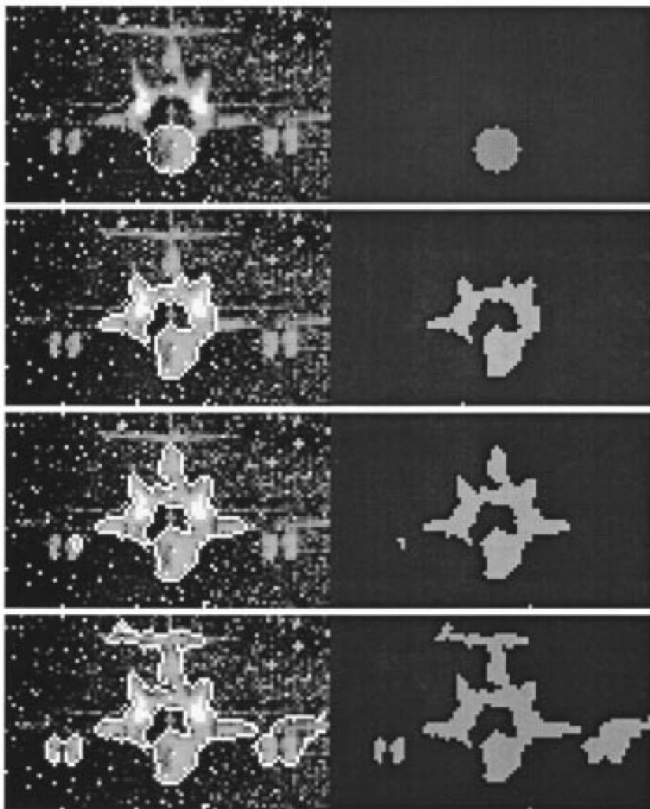
Fig. 13. Detection of the contours of a plane from a noisy image. Size =  $87 \times 53$ ,  $\Delta t = 0.01$ ,  $\mu = 0.17 \cdot 255^2$ ,  $\phi_0(x, y) = -\sqrt{(x - 45)^2 + (y - 39)^2} + 6$ , one iteration of reinitialization, cpu = 2.87 s.
